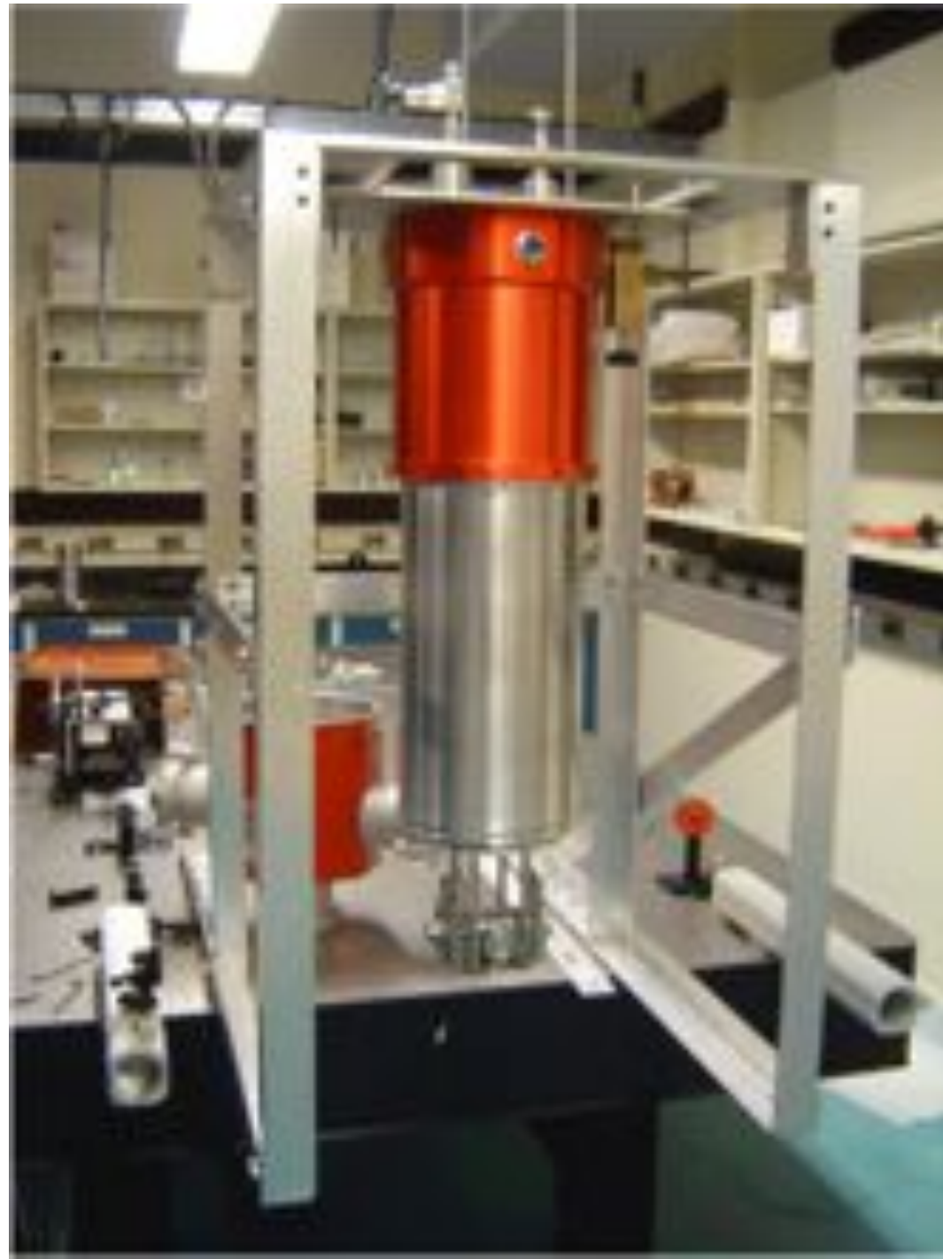
Pumped He-4 system at Yale, with optical access
